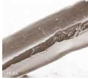
As you can see from these photos, chlorine bleach has caused significant damage to the nylon fiber. Since this fiber is solution dyed, there has been only slight color loss.
